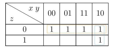
$$f(x, y, z) = x.\overline{y} + \overline{z}$$
