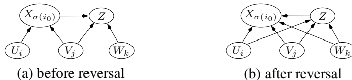
Figure 6.7: The arcs added to the graph by arc (X, Y) 's reversal.
