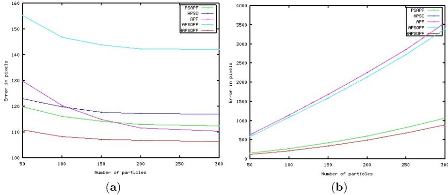
**Fig. 2: Comparison tests for convergence and computation time when tracking the object  $N_a = 4, L_a = 3$ : (a) convergence and (b) computation times (HPSO and our approach give same curves) in seconds.**
