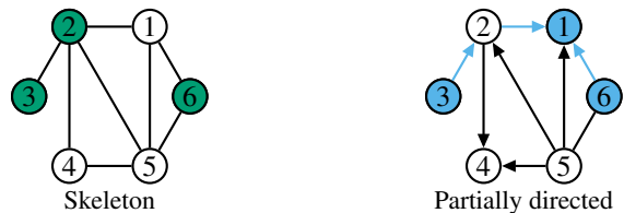
Figure 2: Two scenarios of inconsistent conditional independence: 2 \perp\!\!\!\perp 6 \mid 3 regarding the skeleton, where a path between 3 and 6 that does not go through 2 is expected but missing. And 3 \perp\!\!\!\perp 6 \mid 1 regarding the partially directed graph, where 1 as the common descendant of 3 and 6 is not expected in the separating set.
